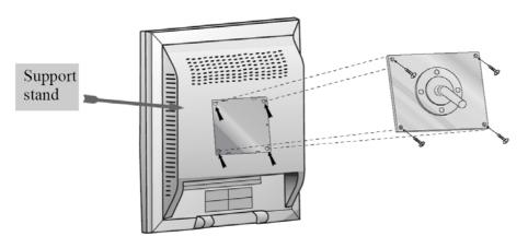
Hole spacing: 100 x 100mm Screw length: 8~12mm
